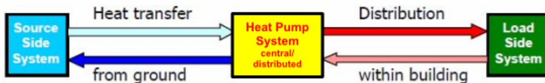
FIGURE 1: THREE PRINCIPAL GEOEXCHANGE SUBSYSTEMS (FROM GEOEXCHANGE BC, PROFESSIONAL GUIDELINES FOR GEOEXCHANGE SYSTEMS IN BRITISH COLUMBIA, 2014)
