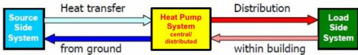
FIGURE 1: THREE PRINCIPAL GEOEXCHANGE SUBSYSTEMS
